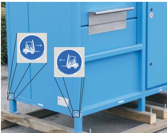
fig. 5.1-1 Lift point markers
